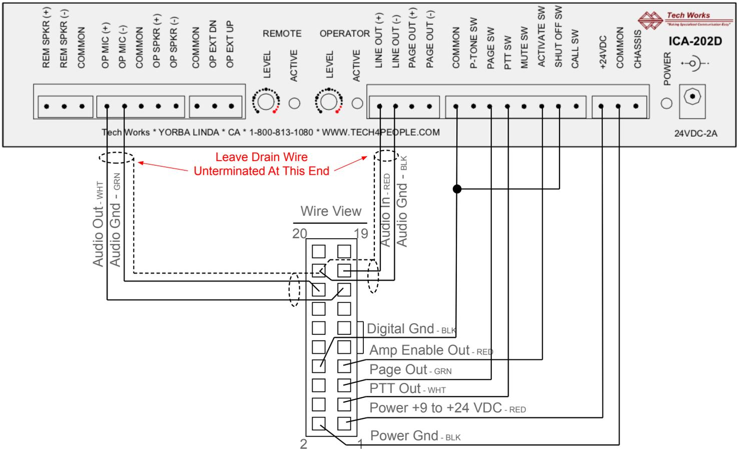
Simplex Amplifier Wiring Diagram
